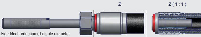
Fig.: Ideal reduction of nipple diameter
