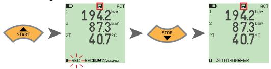
The file name is incremented for each sequential measurement. The files are stored with date and time.
