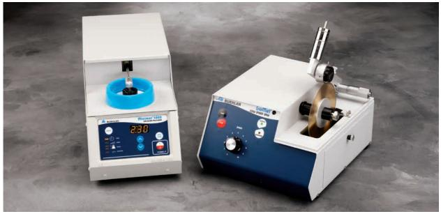
The IsoMet<sup>®</sup> Low Speed Saw is an excellent companion to the MiniMet<sup>®</sup> 1000 Grinder/Polisher including when low deformation sectioning is required prior to polishing.
