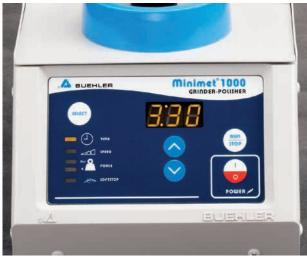
Control Panel features touch-pad controls and LED displays of all grinding/polishing parameters.
