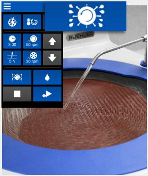
On the main screen, press and hold the "Rinse and Spin" button to begin the cycle.
