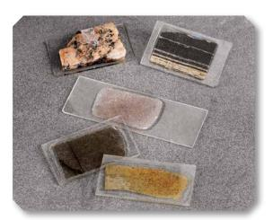
Mineral samples re-sectioned and thinned to 30µm.
