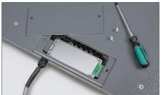
Easy levelling of the weighing bridge as well as access to the junction box from above
