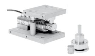
The SHBxR foot assembly is an ideal solution for low and medium capacity platform scales. The SHBxR mount and foot are based on a rocker pin design, combining excellent load introduction to the transducer with an overall low profile.
