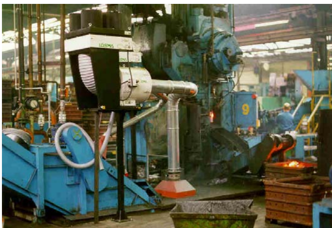
Air filter for oil mist model Aspirofilter AS 8 DC, complete with electrostatic after filter model Synthesis and final filtration stage at activated carbons for smoke and odours model Microfilter CA on hot moulding machine. TRW, Germany
