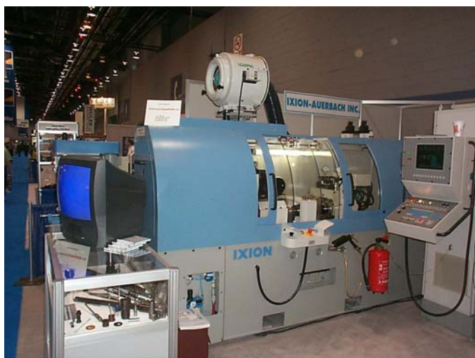
Air filter for oil mist model Aspirafil AS 4 on IXION drilling machine.
