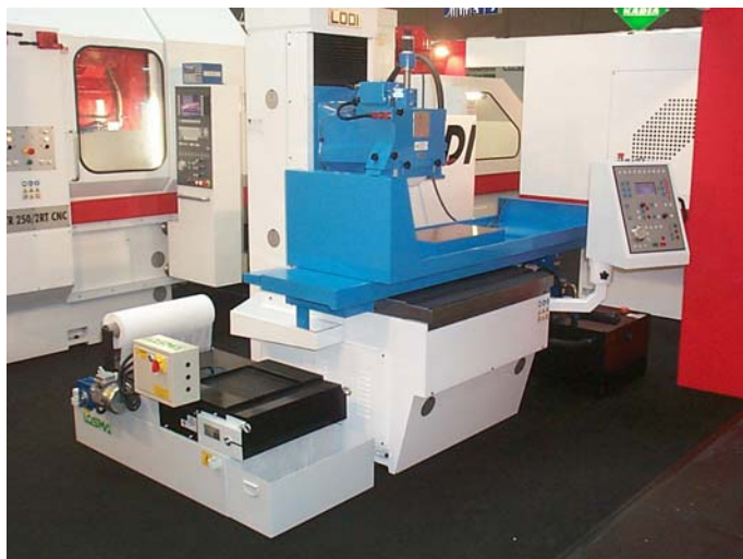
Coolant filter model Detex 50, Paper media on grinding machine LODI.
