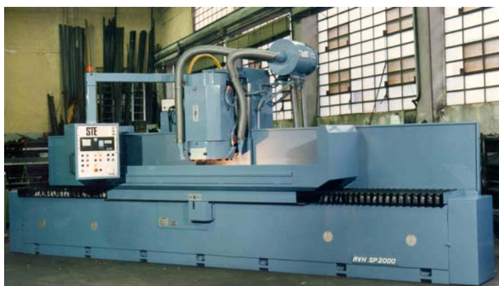
Air filter for oil mist model Aspirafil AS 5 L with two suction hoods on grinding machine. Stefor, Italy
