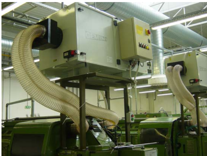
GEMINI ELECTROSTATIC WITH DOUBLE SUCTION PIPING
