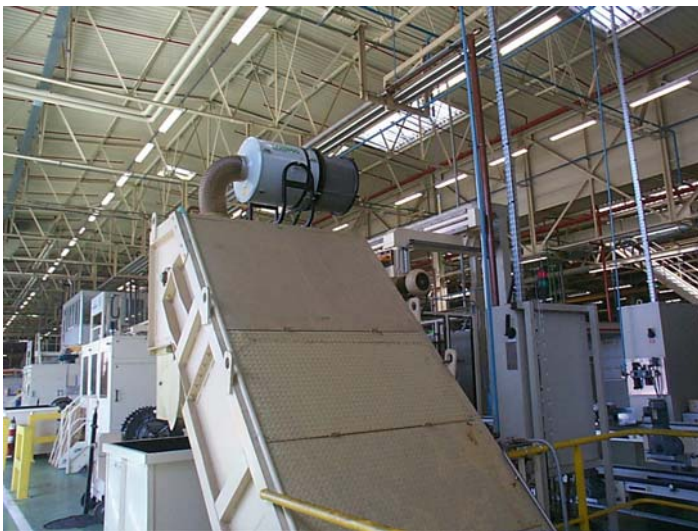
Air filter for oil mist model Darwin 3000 in horizontal position, complete with cartridge after filter model Clipper on filtration system . Renault plant, France.
