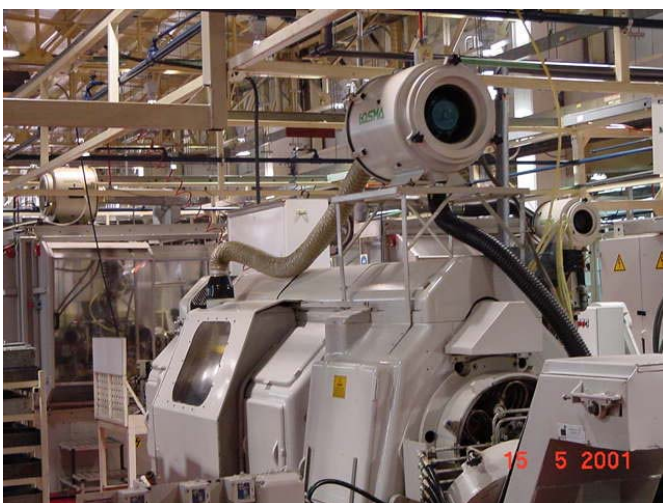
Air filter for oil mist model Aspirofiler AS 4 DC mounted on special support, on turning machine.
