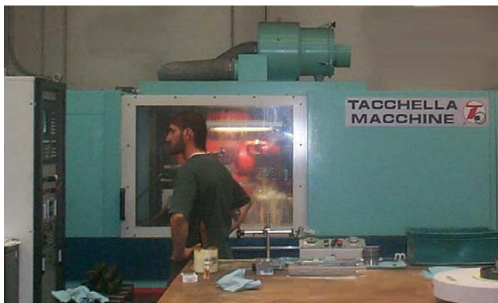
Air filter for oil mist model Aspirafil AS 5 L on TACCHELLA grinding machine.
