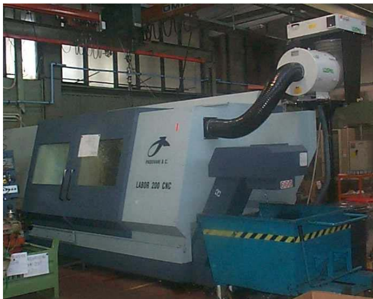
Air filter for oil mist model Aspirofiler AS 8 DC complete with electrostatic after filtration stage model Synthesis on Padovani turning machine.
