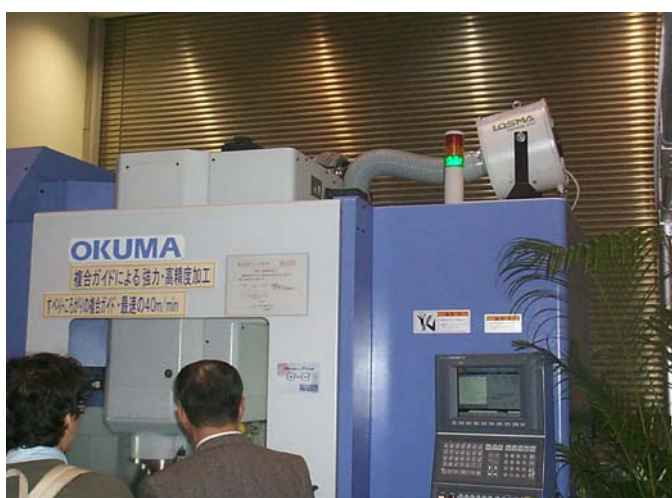
Air filter for oil mist model Darwin 600 in horizontal position on vertical turning machine OKUMA.
