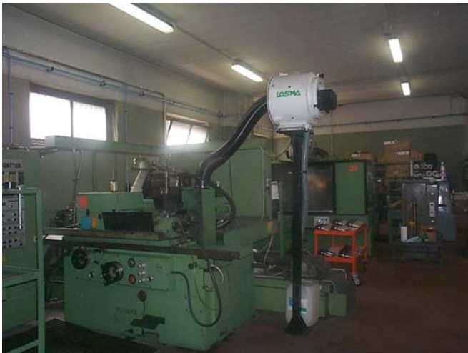
Air filter for oil mist model Aspirofiler AS mounted on universal vertical stand and suction hood directly to the working area on universal grinding machine.
