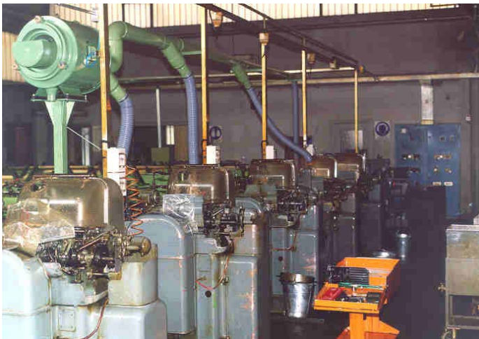
Air filter for oil mist model Aspirofiler AS 4 DC on four small turning machines with transparent suctions hoods.
