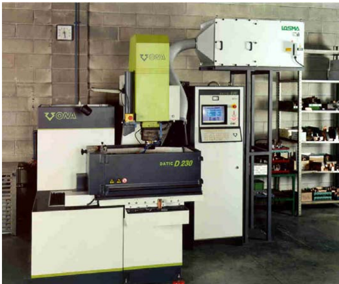
Air filter for smokes, oil mist and micro-mists, model SIRIUS 800, on spark erosion machine a tuffo ONA
