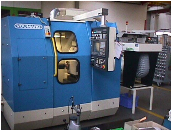
Air filter for oil mist model Aspirofiler AS 4 DC complete with electrostatic after filtration stage model Synthesis E 2000 on grinding machine VOUMARD. Per interni
