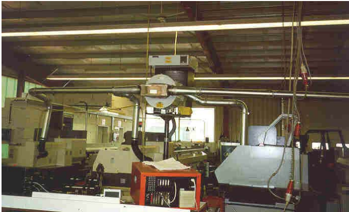
Air filter for oil mist model Aspirofiler AS 8 DC complete with electrostatic after filtration stage model Synthesis E 2000 M on three turning machines.
