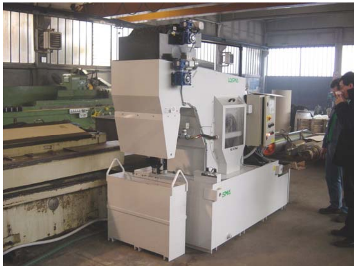
SPRING F4 MAGNETIC PRE-FILTER SELF-CLEANING DRUM FILTER
