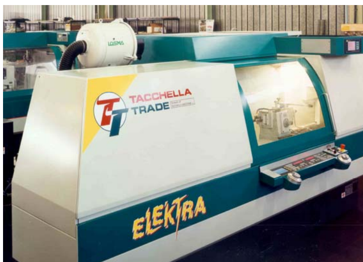
Air filter for oil mist model Aspirafil AS 3 with air deflector on Tacchella grinding machine.
