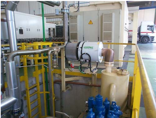
Air filter for oil mist model Darwin 3000 in horizontal position, complete with cartridge after filter model Clipper on filtration system . Renault plant, France.
