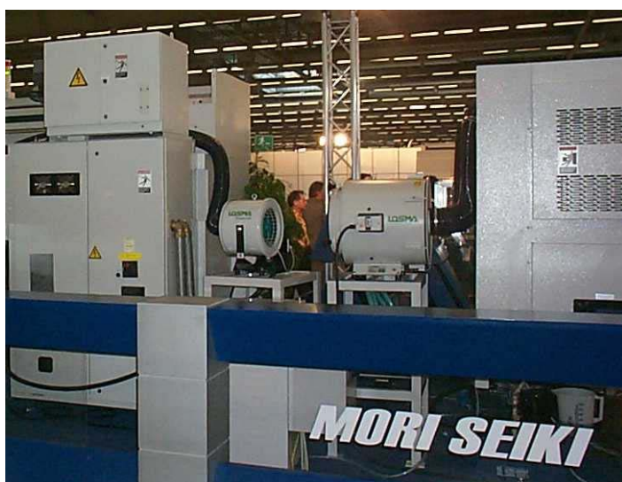
Set of air filterS for oil mist model Aspirofiler AS 4 DC and Darwin 600 in horizotal position on MORI SEIKI machining center.
