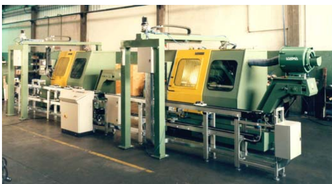
Air filter for oil mist model Aspirofiler AS 4 DC with air deflector, on turning machine.
