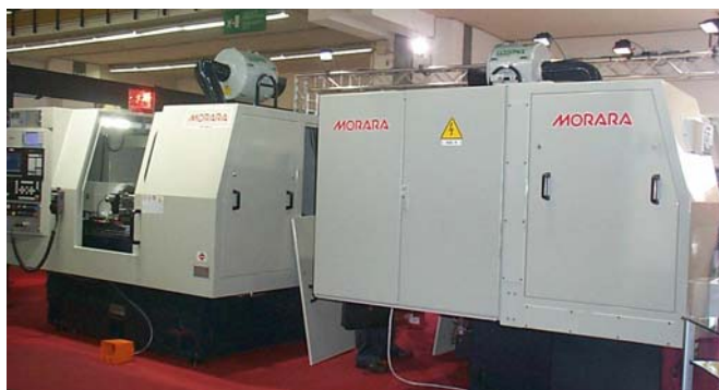
Air filter for oil mist model Darwin 2000 in horizontal position with air deflector on Morara grinding machine Cabinata per interni.
