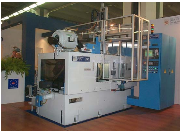
Air filter for oil mist model Aspirofiler AS 5 L on Bocca&Malandrone no centers grinding machine.
