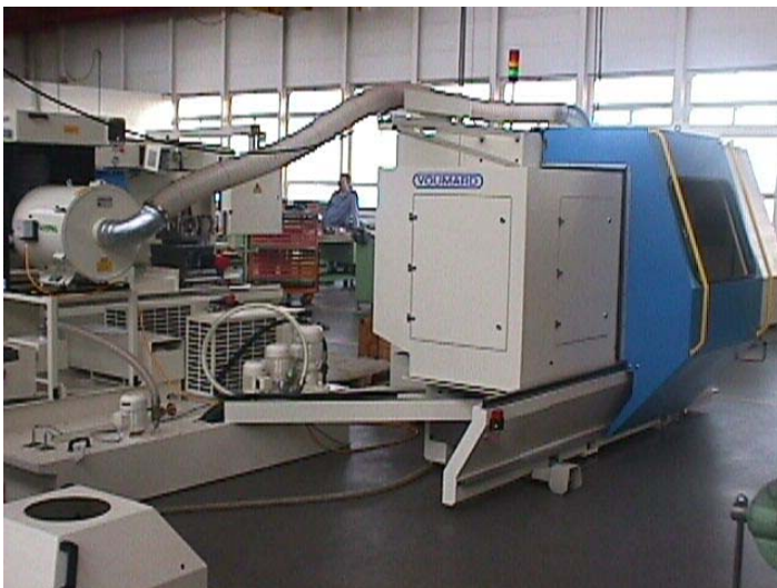
Air filter for oil mist model Aspirofiler AS 4 DC on grinding machine VOUMARD. Per interni
