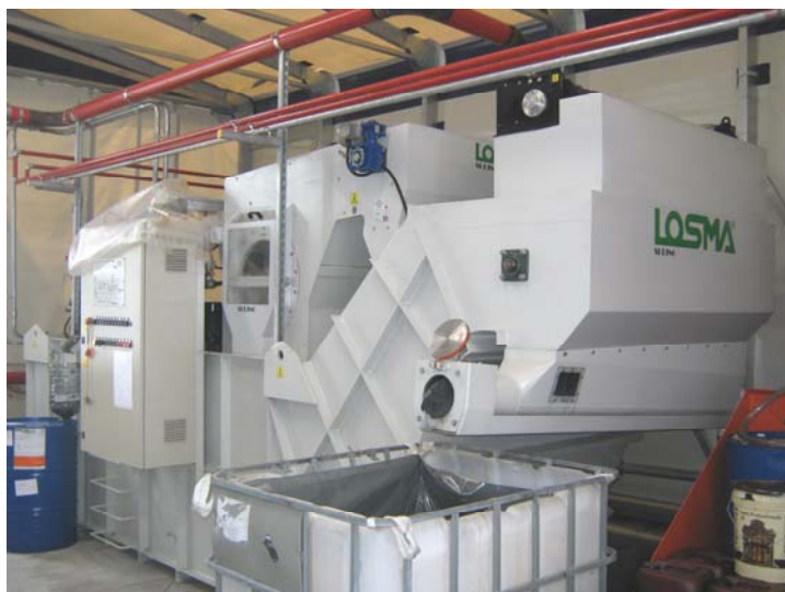
SPRING F7 MAGNETIC PRE-FILTER SELF-CLEANING DRUM FILTER MUD COMPACTOR
