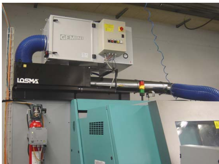
GEMINI ELECTROSTATIC EL WITH GUARD PRE-FILTER
