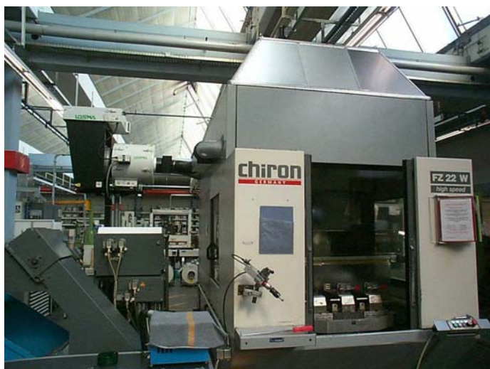
Air filter for oil mist model Aspirofiler AS 8 DC complete with electrostatic after filtration stage model Synthesis on universal milling machine CHIRON at Festo, Germany
