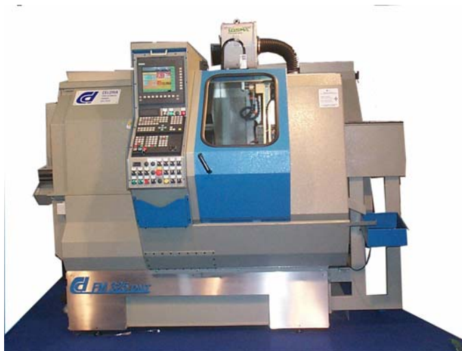
Air filter for oil mist model Darwin 600 in horizontal position with air deflector on CNC CELORIA turning machine.
