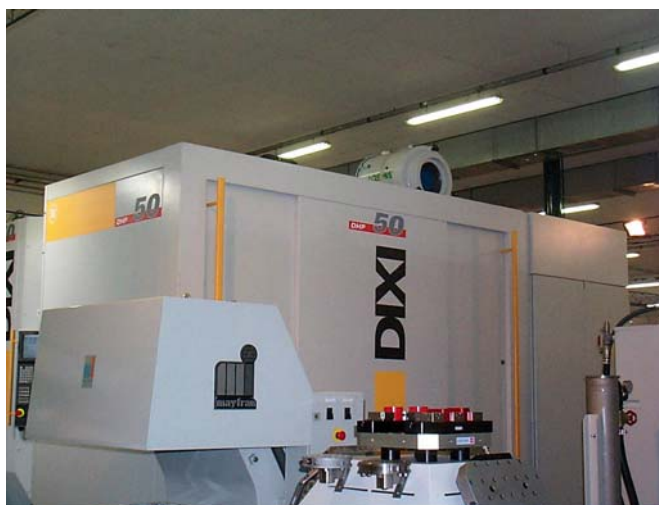
Air filter for oil mist model Aspirafil AS 4 DC on DIXI machining center.
