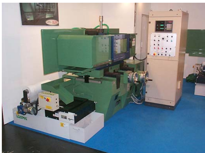
Coolant filter model Detex 50, Paper media on grinding machine STEFOR
