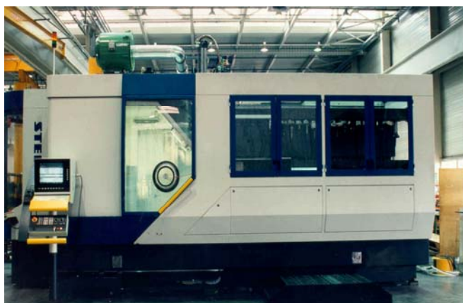
Air filter for oil mist model Aspirofiler AS 4 on STEINEL machining center.
