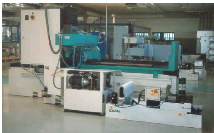
Coolant filter model Detex 100, Paper media on grinding machine.
