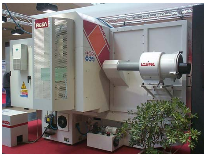
Air filter for oil mist model Aspirafil AS 5 L with air deflector on ROSA grinding machine.
