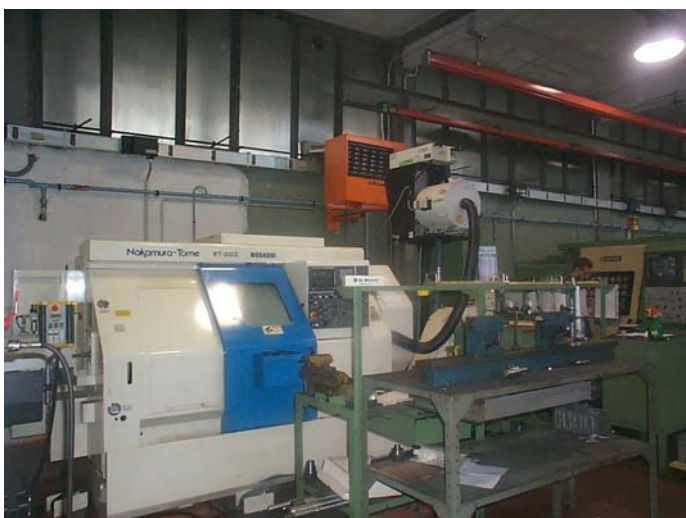
Air filter for oil mist model Aspirofiler AS 3 DC complete with electrostatic after filtration stage model Synthesis E 1000 on Nakamura neat oil turning machine.
