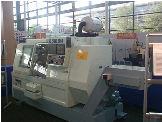
Air filter for oil mist model Aspirafil AS 4 on Biglia turning machine.
