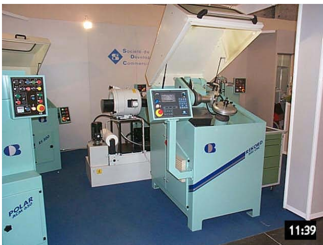
Coolant filter model Detex 50, Paper media and air filter for oil mist model Aspirofilter AS 1 on a sharpening machine Businaro.
