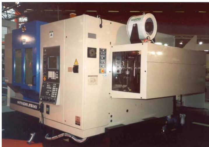
Air filter for oil mist model Darwin 600 in horizontal position, on machining center HITACHI SEIKI
