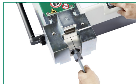
Tooling head for 37° tube flaring based on settings manually defined by the operator
