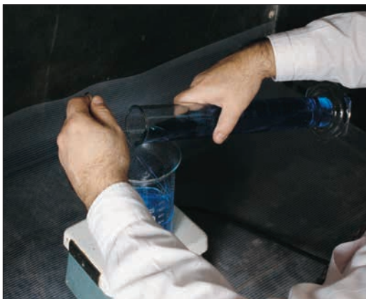
Figure 71. When mixing etchants, use a magnetic stirring plate with a magnetic bar for stirring. Slowly add the liquid ingredients to the solvent by dripping them down a glass stirring rod. If the solution is more dangerous than this one, wear protective gloves and use a face shield. If mixing generates substantial heat, it is a good practice to place a cooling jacket around the beaker.
