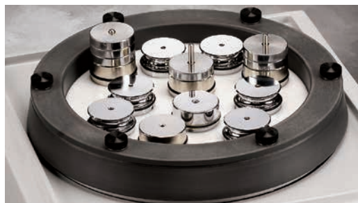
Figure 33. Preparation with sample holder and adding weight.
