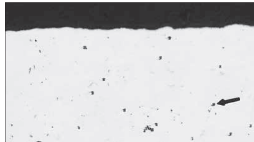
Figure 19. Pitting (arrow) on the surface of a cold-drawn brass (Cu-20% Zn) specimen (100X)
