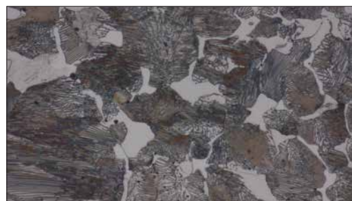
Normalized carbon steel shows coarse ferritic-pearlitic (grains with lamellar cementite) structure. Etched with 3% Nital (200X).
