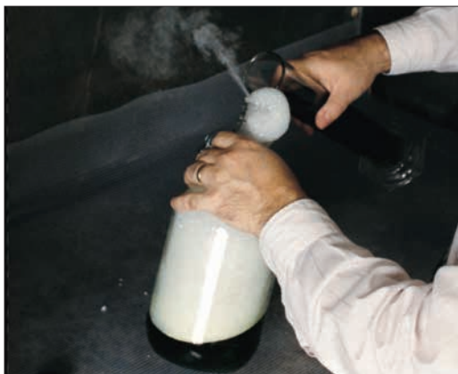
Figure 72. Illustration of a bad mixing practice. The acid ingredient was poured into an empty acid bottle and the solvents were added without stirring or cooling. The solution may erupt in the metallo-grapher's face at any moment. It is recommended to keep the hands clear of the area and remove rings.
