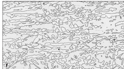
Figure 41. Microstructure of a duplex stainless steel revealed by electrolytic etching with (c) aqueous 60% HNO 3 (1 V DC, 20 seconds); with (d) aqueous 10% oxalic acid (6 V DC, 75 seconds); with (e) aqueous 10% CrO 3 (6 V DC, 30 seconds); and, with (f) aqueous 2% H 2 SO 4 (5 V DC, 30 seconds) at 200X.
