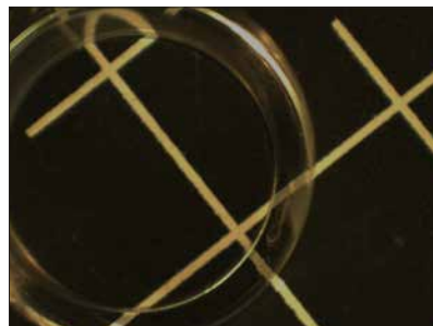
Quartz tube after 6µm polish.
