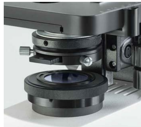
Mounted phase contrast condenser
